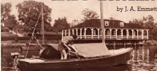
Keeping a canvas cover over the open cockpit of a boat when not in use is an important protection against rot. Salt water is anti-rot, but rain water settling in the bilge may quickly start it.
